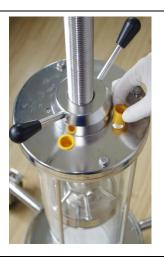
c. Before use, tighten the nut of feed port to avoid the risk of leakage (if the sealing ring of feed port is damaged, it needs to be replaced in time). If external pipe connection is required, place gasket evenly between pipe and cylinder, then lock it with clamp and tighten it.
