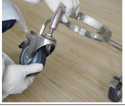
c. After fixing the end-piece, the white guide ring is installed in the end-piece card slot.
