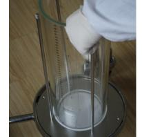
c. Buckle the upper O-ring into the flange.
