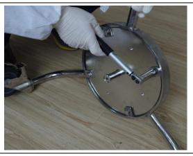
d. Place the support net plate flat in the center of the end-piece.
