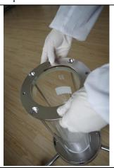
e. Put in the gasket and tighten with a torque wrench.
