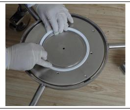
e. Install the lower filter net.
